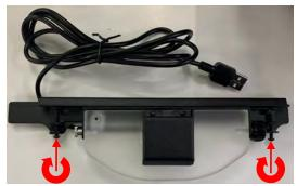
2. Separate the Bracket from the Camera
