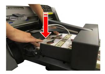
4. When using Blowers, adjust the rotation speed of Blowers and the width of Side Media Guide So that the media slightly rises.
