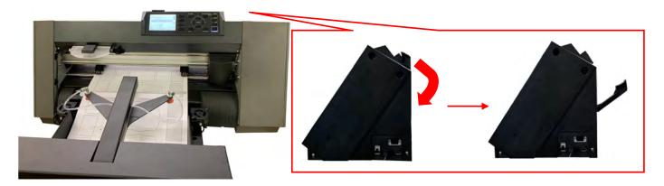
2. Pull out the tip of media to the front of Push Roller on the CE7000-40.
