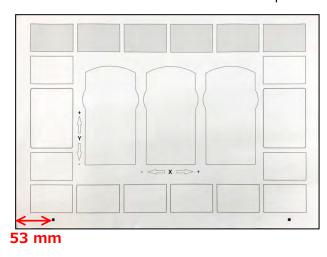
9. Make sure that the "Cutter ready" is displayed on the bottom of the iMark Plus software window, and then click the "Cut Test" button to perform the cut test to the Test Cut sheet.
