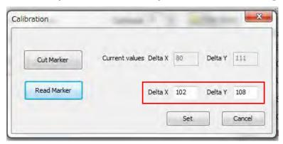
7. Click the "X" button on the upper left on the Calibration window to close it, and remove the calibration sheet from the CE7000-40 and finish the calibration.
