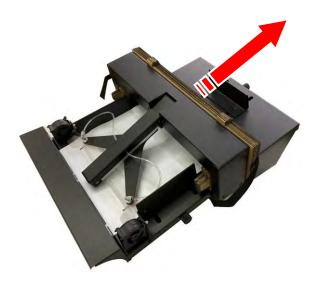
13. Detach the two cushioning materials under the Arm from the F-Mark2.
