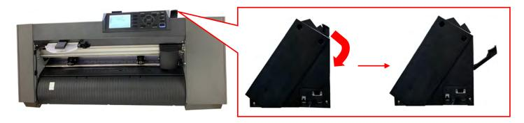
2. Move the left side Push Roller onto the leftmost Grid Roller as shown in picture below. And adjust the position of the left side Push Roller so that the right edge of the brass part on the Push Roller is align with right edge of Grid Roller as show in picture below.
