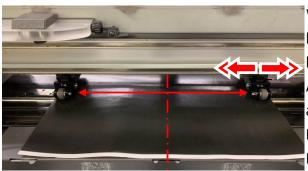
When loading the calibration sheet into the CE7000-40, load the calibration sheet so that the it is centered between the left and right Push Rollers.
