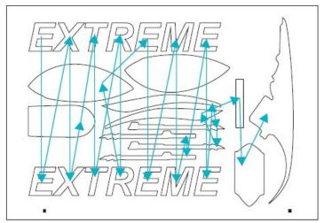
When "Cutting direction sorting" is unchecked, the order of cutting is reversed order of drawing order of cut contour shape graphics as shown below figure.
