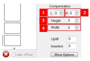
The printed images with digital printer are often distorted. The iMark Plus software uses the optical camera to detect the crop marks to corrects distortions in the printed images near the crop marks and to corrects the cutting position.
