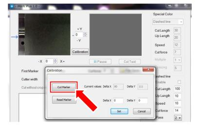
5. Peel off a small square cut by the CE7000-40 from the Calibration Sheet so that the white square can be see.
