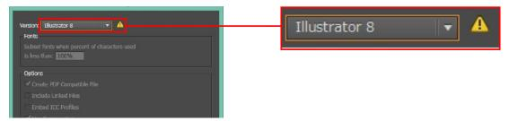
When loading the cut contour shape graphics file which has not been saved in Illustrator 8 format into the iMark Plus software, the massage of "Graphics file not saved correctly" will be displayed and file can not be loaded into the iMark Plus software.
