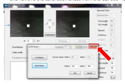
8. After calibration is finished, perform the "Test Cut" to check the calibration of the F-Mar2 is correctly.
