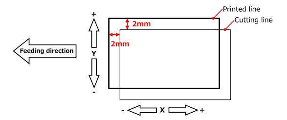
1. Input "-20" into the X, and input "20" into Y.
