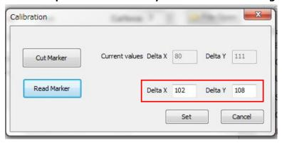
7. Click the "X" button on the upper left on the Calibration window to close it, and remove the calibration sheet from the CE7000-40 and finish the calibration.
