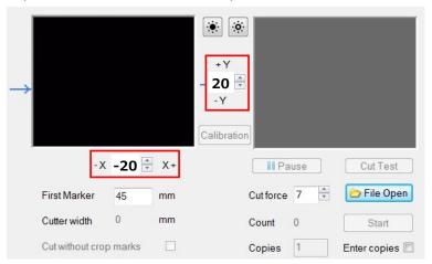
2. And then click the "Cut Test" button to perform the cut test, and confirm the cutting position.
