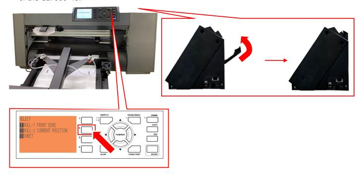
3. Set the Cutter Plunger to the back side (for Half Cutting) of the Tool holder on the CE7000-40.
