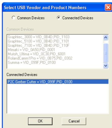
**10** Choose the connected USB plotter from the Connected Devices list (or the Common Devices list if it is a plotter in that list) and click OK. This will load the USB information (Vendor ID and Product ID) for the plotter into OMEGA. Click OK.
